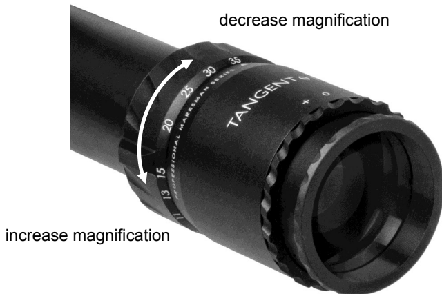
Fig. 2c Increase magnification by turning the ring counter-clockwise. Decrease by turning clockwise.
