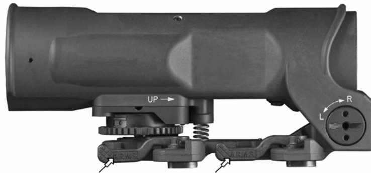
To fully disengage the ARMS levers, rotate them to a position 90° with respect to the sight body. Close levers to lock sight onto rail.
