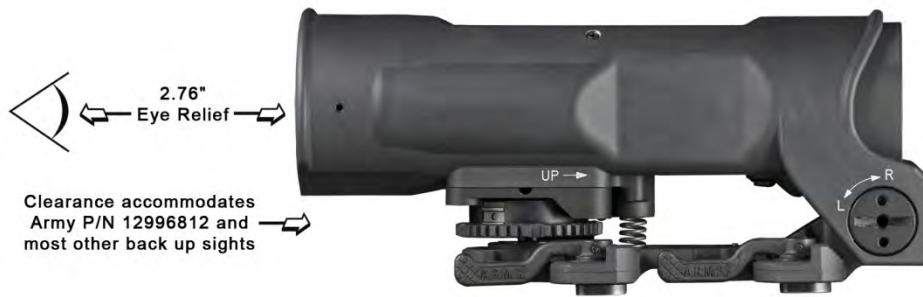
Figure 1-2 Long eye relief facilitates use with most back up iron sights.
