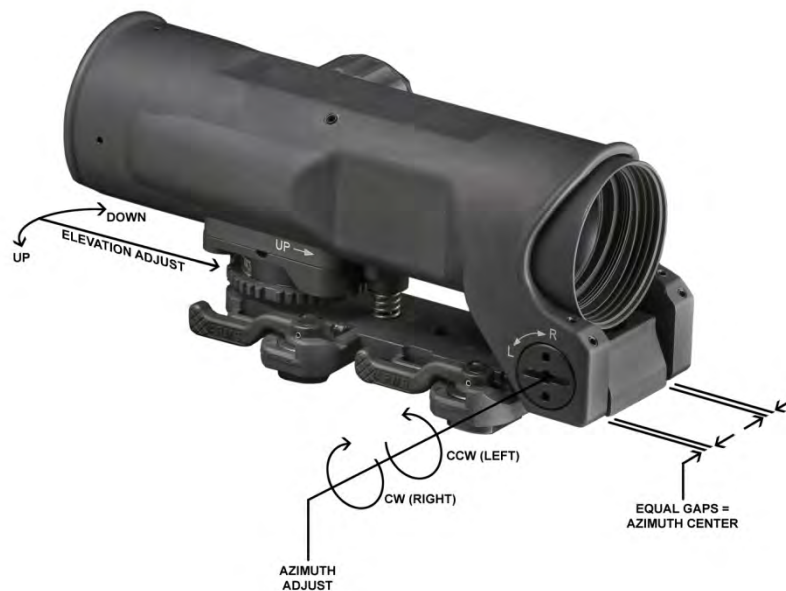
Figure 3-1. Azimuth (Windage) Zeroing Adjustment
